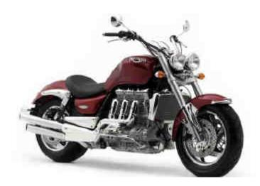
The Rocket III motorcycle is one of a range of cruiser bikes designed and manufactured by Triumph Motorcycles Ltd of England. The Rocket III is the largest production motorcycle in the world. It has a fuel injected, twelve valve, 3 cylinder in-line engine of 2294cc cubic capacity which gives 147ft lbs of torque at 2500 rpm. This triple cylinder engine arrangement is special to Triumph.
