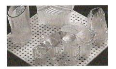
**1992 -** DTM produces first SLS (selective laser sintering) machine. This machine is similar to SLA technology but uses a powder (and laser) instead of a liquid.
