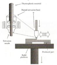
The main difference between the first technique and two others is that selective laser sintering (SLS) and fused deposition modelling (FDM) use melting or softening material to produce the layers
