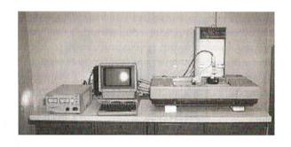
Charles Hull, later the co-founder of 3D Systems, invents stereolithography, a printing process that enables a tangible 3D object to be created from digital data. The technology is used to create a 3D model from a picture and allows users to test a design before investing in a larger manufacturing program. Stereolithography (SLA) – was patented in 1987
